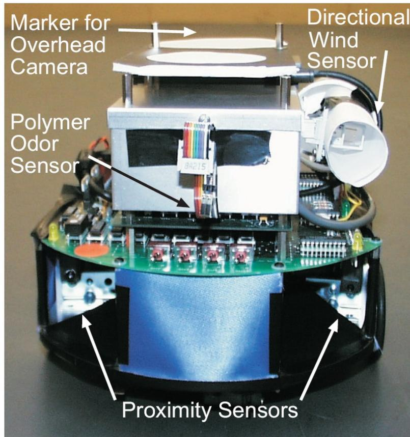
Figure 4 - Moorebot robot fitted with a polymer odor sensor (electronic nose), and other sensors. (Source: [http://www.coro.caltech.edu/people/alcherio/papers/Robotica\\_03.pdf](http://www.coro.caltech.edu/people/alcherio/papers/Robotica_03.pdf))
